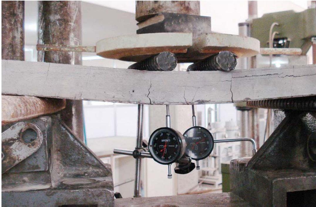
Fig. 6: Testing Of Specimens Under Two Point Loads.
